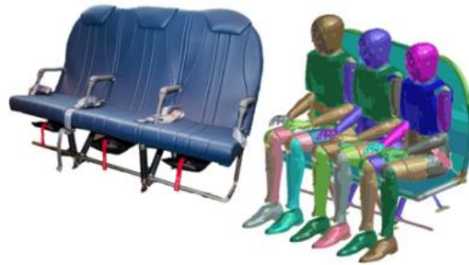
Expliseat's Titanium Seat (left) seat virtual prototype (right).
